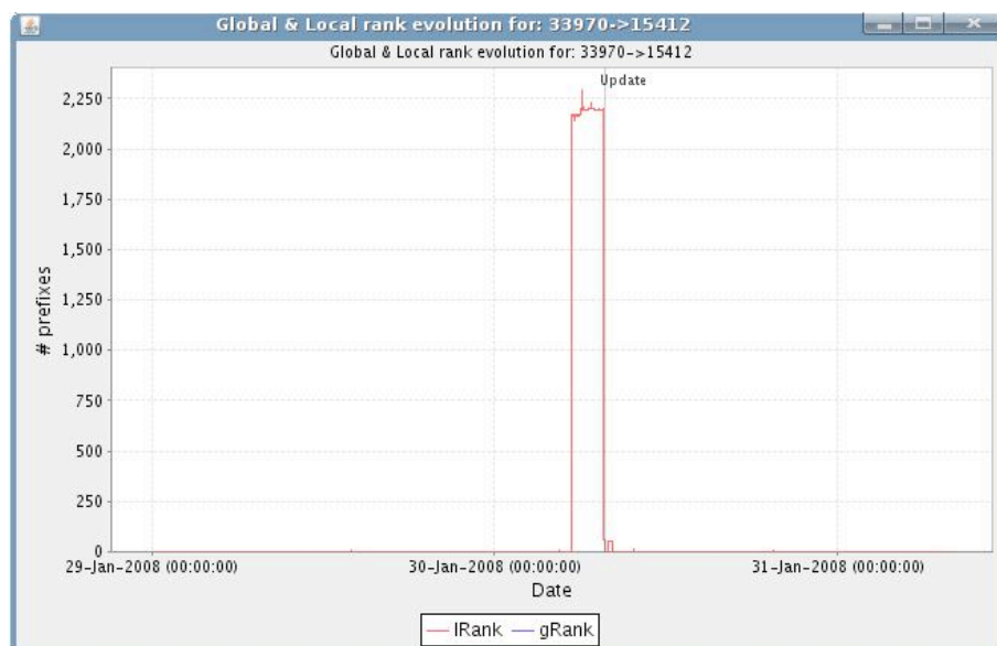
Figure 11: AS33970 (OpenHosting) temporarily routed a large set of prefixes through FLAG Telecom (AS15412). It took more than two hours to return to the previous usage level.
